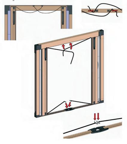
■ Insert the two pleated screen packs into the tracks. ■ Move the two screen packs towards their respective starting profiles. ■ Insert the two screen packs into the starting profiles until they are snap-locked into place.
